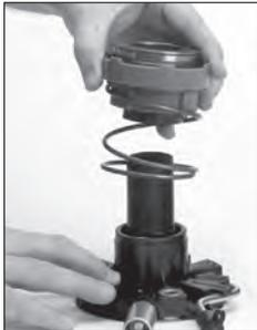
Seat the new release bearing assembly on the slave cylinder spring and install the assembly on the slave cylinder.
