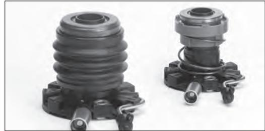
This procedure provides instruction for bearing installation on slave cylinders that include a spring boot assembly and plastic spacer.
