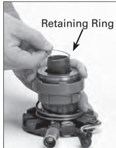
Press down on the bearing to install the new retaining ring, included in the clutch set.
